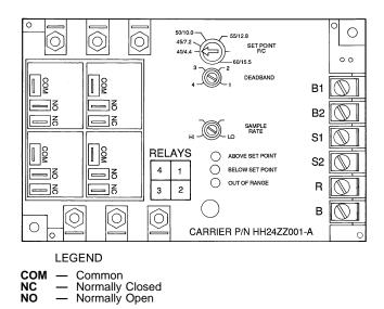
Fig. 21 — Temperature Controller
